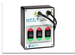
Designed to provide a fast, safe and reliable operational verification of Dielectric Withstand (hipot) and Ground Continuity Testers between calibration cycles. It allows the operator to check the result of the three failure modes encountered in production hipot and ground circuit testing (open ground, high leakage current, and dielectric breakdown) separately or in any combination to verify proper test equipment operation.
